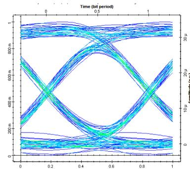
**Figure 8:** Eye diagram of downstream signal at ONU in WDM-PON with two cascaded AWGs
