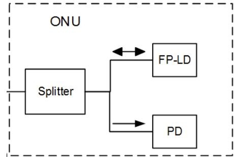
**Figure 7:** ONU part in WDM-PON with two cascaded AWGs
