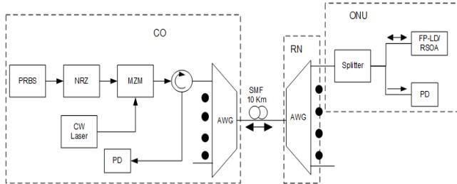
**Figure 12:** Architecture of WDM-PON showing colorless sources based on RSOA or FP-LD with two cascaded AWGs.
