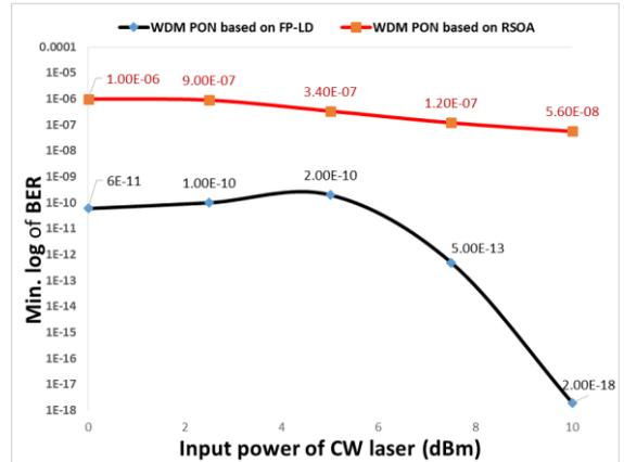
**Figure 13:** WDM PON based on RSOA versus WDM PON based on FP-LD in the results of upstream BER when input power of CW laser is increased.
