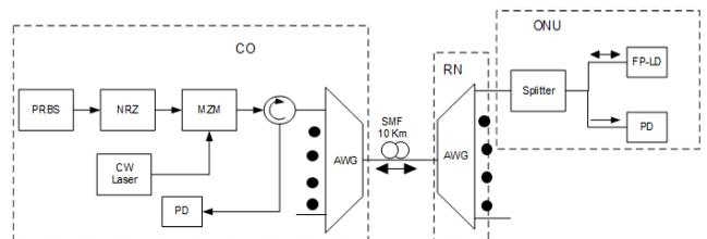
Figure 5: Block diagram of the proposed bidirectional PON system model
