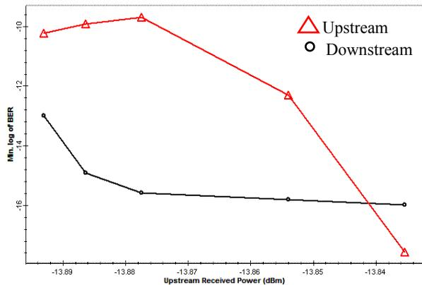
**Figure 10:** Min. log of BER versus upstream received power at CO for downstream and upstream signals in WDM-PON with two cascaded AWGs
