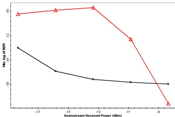
**Figure 9:** Min. log of BER versus Downstream received power at ONU for downstream and upstream in WDM-PON with two cascaded AWGs
