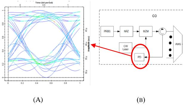
**Figure 6:** (a) Eye diagram for upstream signal at CO in WDM-PON with AWG at RN, (b) The transceiver at CO
