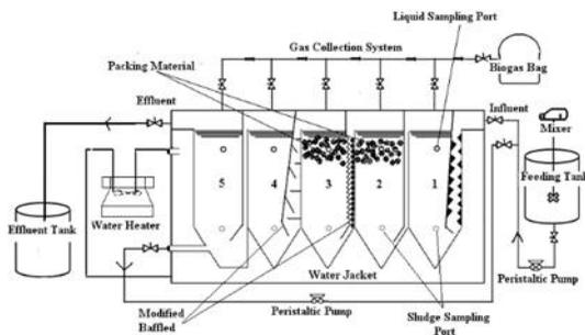
Figure 1: Laboratory Scale Modified Anaerobic Hybrid Baffled (MAHB) Reactor
